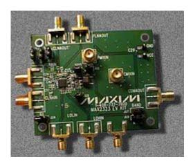
Objective: To develop an application circuit for using this dual-band triple-mode CDMA front-end IC, employing the PCS-band downconverter for the 2.5GHz LEO satellite channel and the cellular-band downconverter for IS-95 CDMA.
